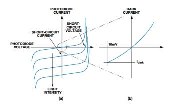
Figure 2. Typical Photodiode Transfer Function
