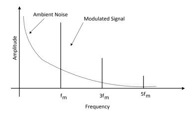
Figure 9. Chopping the Input Signal Moves the Information to the Chopping
