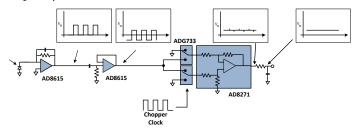
Figure 10. Synchronous Detection Circuit
