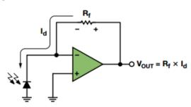
Figure 1. Simple Transimpedance Amplifier Circuit
