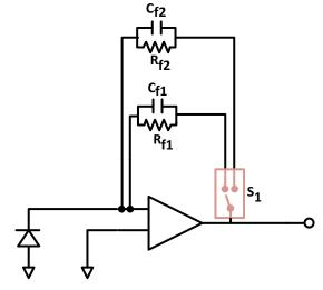
Figure 7. The Concept of a Programmable Gain Photodiode Amplifier
