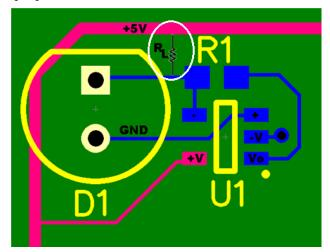
Figure 3. Photodiode Layout with Leakage Path
