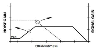
Figure 6. The Noise Gain of a Photodiode Amplifier Increases at Higher Frequencies
